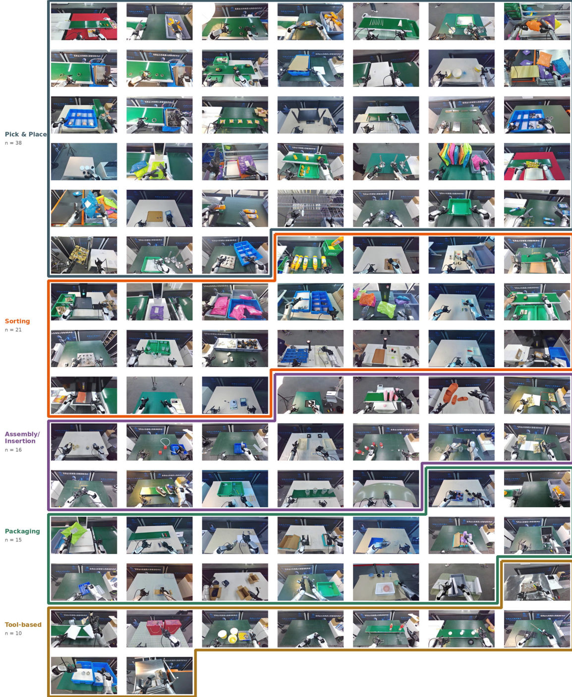
Figure 2. Task-category composition of the 100-task domain-specific retraining dataset, with representative head-camera frames from each category. Every frame comes from the same Kuavo4pro embodiment.
